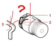
> **For regular threads:** Hold the thread with both hands and insert it into the guide (1) from below. Feed the thread from right to left through the thread take-up lever (2). Feed the thread through the guide (1) from above.
